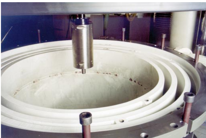
Burst proof enclosure consisting of 3 steel rings
