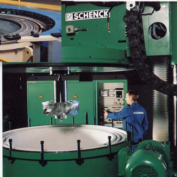
Inducer disc installed in a Spin-Test System BI 4 U
