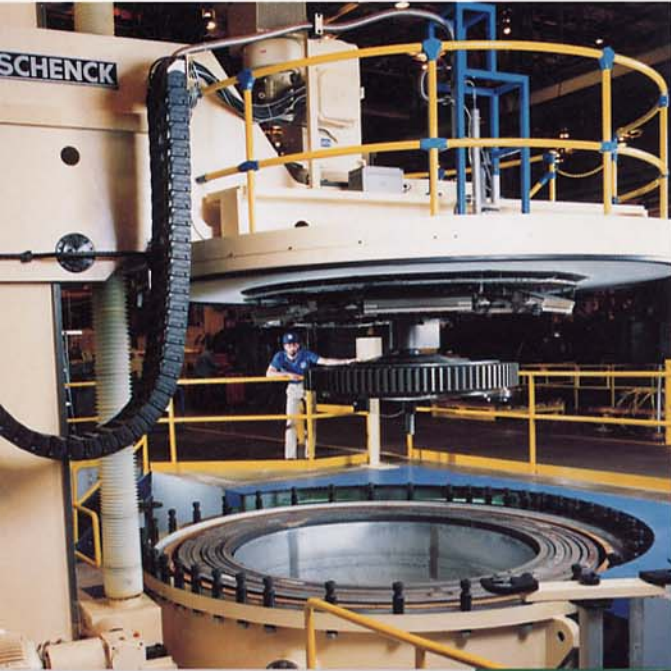
Gas turbine disc prepared for a hot and cold test in a Spin-Test System BI 7 U
