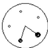
If you can only fit the balancing weight to the rotor at certain positions (e.g. on the blades of a fan), select the correction mode 'Fixed location'. Then enter the 'Number of locations' on the rotor. The Smartbalancer calculates two weights in the balancing runs which must be fitted at two of the specified positions. Position or blade #1 corresponds to the 0° position and should be set up as the reference mark for the reference pick-up.
