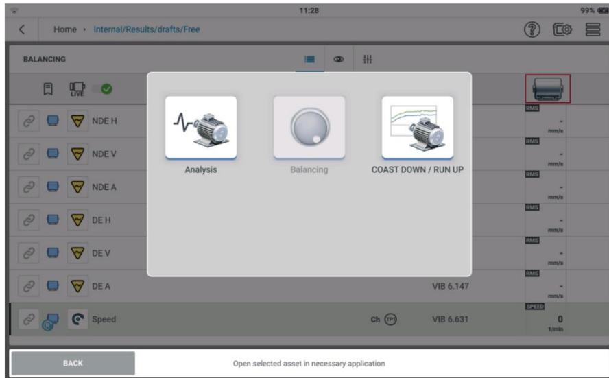
In this example, the available applications are **ANALYSIS** and **COAST DOWN/RUN UP**. This is because the application change started from the balancing application. Thus, the icon is shown grayed out. Note: if advanced analysis is not installed in the unit this icon will not appear.
