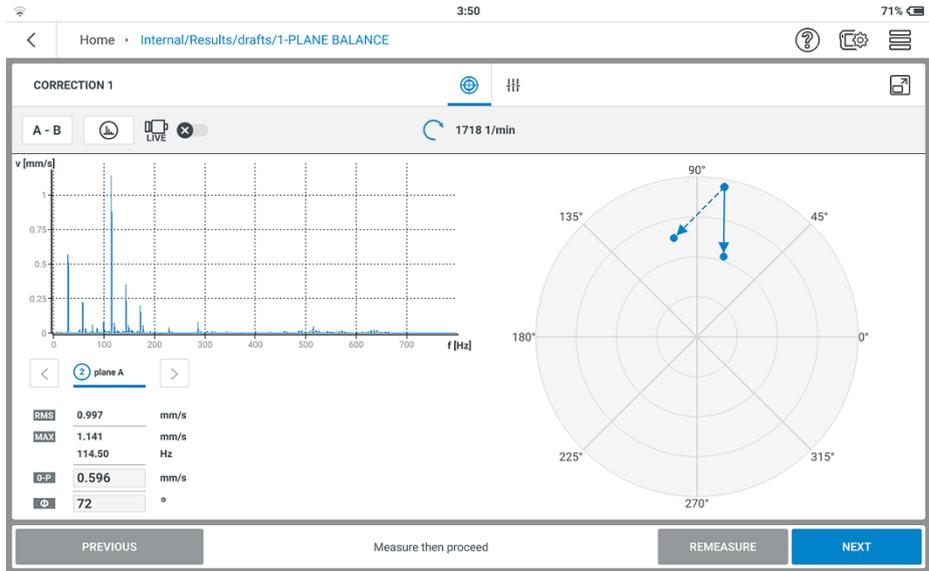
In the correction runs, the Smartbalancer checks whether the unbalance has been reduced sufficiently from one run to the next.
