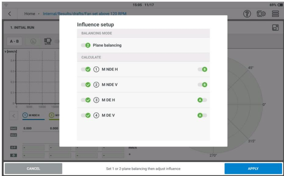
The SmartBalancer will use the data received from all sensors connected to calculate the recommended correction weights in order to optimize the balance for locations monitored.
