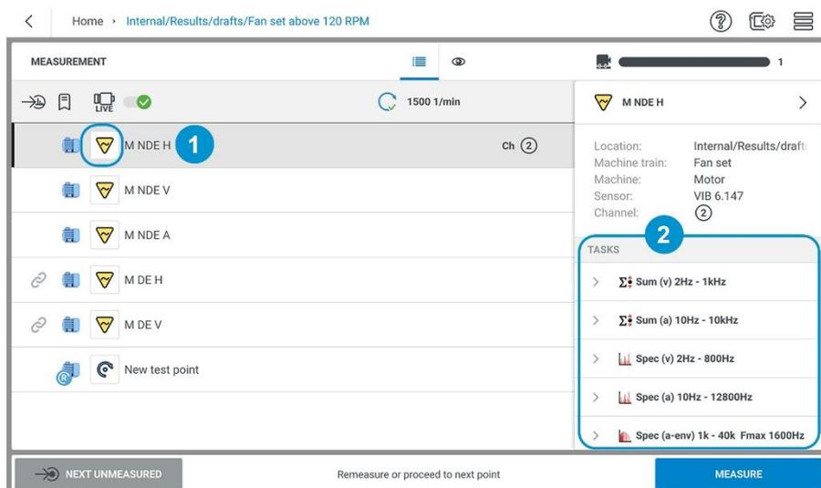
Tap the parameter icon (1) to see the applied measurement task (2) for the selected location.
