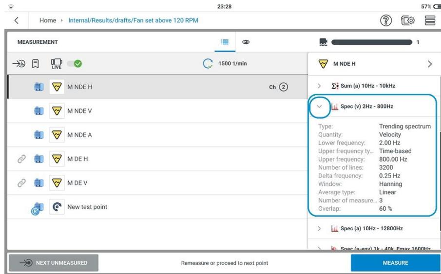
To see the details of any of the applied measurement tasks, tap the related task drop-down menu.
