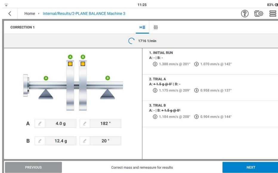
Continue the correction runs until the residual unbalance is within the tolerance range.
