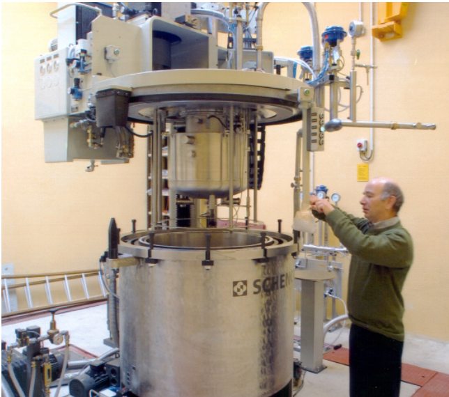
Spin test system with cryo service for low-temperature tests
